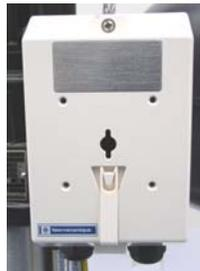
Remove security tab, and undo the two screws securing the isolator switch housing, and remove housing.
