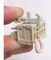
Pushing down on tool causes the pin of the anchor to operate the jaw mechanism. The jaw opens allowing the wire to be inserted.
