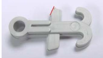
The anchor tool is double sided, to suit the two styles of terminal blocks used in the terminal box. The anchor tool requires a slight modification for it to work correctly with the white terminal blocks. Trim off a small amount of material from the peg as shown.
