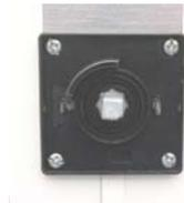
Remove four screws securing isolator switch bezel, and remove bezel.
